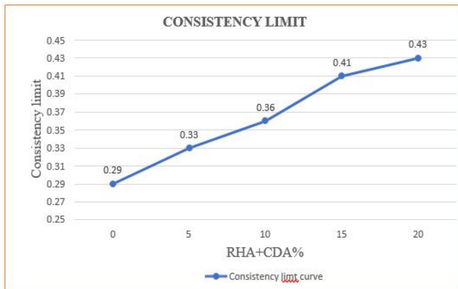
Fig. 3: Consistency curve for RHA+CDA concrete mix
