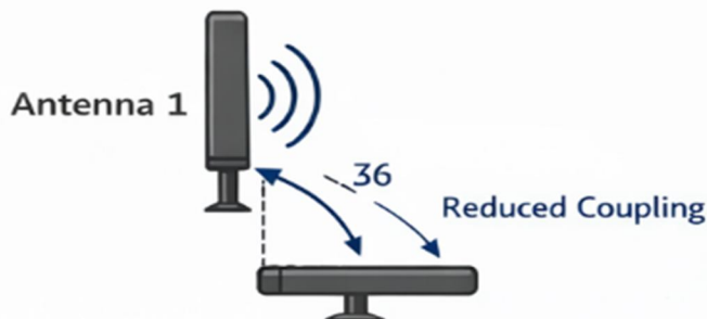
Fig 2.5: Orthogonal Antenna Configuration for Improved Isolation
