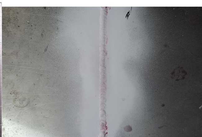
Fig 3.9: DP Testing after applying developer
