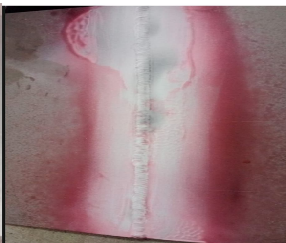
Fig 3.5: DP Testing after applying developer
