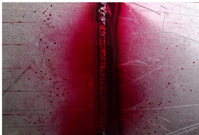
Fig 3.8: DP Testing after applying penetrant
