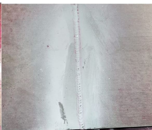
Fig 3.7: DP Testing after applying developer
