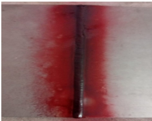
Fig 3.4: DP Testing after applying penetrant
