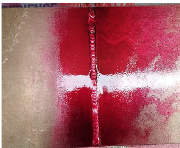
Fig 3.6: DP Testing after applying penetrant
