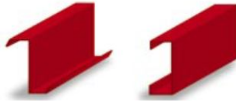
Figure 2: Cold-Formed “Z” And “C” Structural Members.
