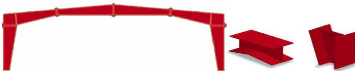
Figure 1: Built-Up "I" Shaped Primary Structural Framing Members
