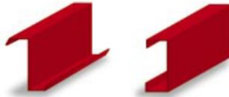
Figure 2: Cold-Formed “Z” And “C” Structural Members.
