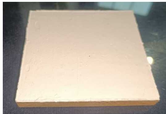
Fig: Teak Wood coated with Intumescent Coating
