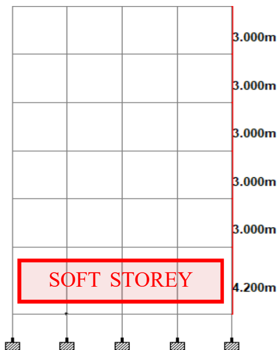
BARE FRAME SOFT STOREY AT GROUND
