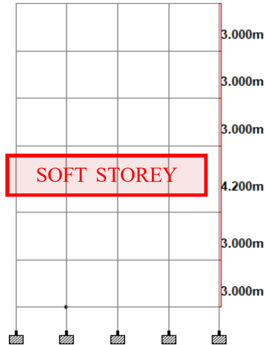
FIG. 4. 5: Soft Storey AT 2 ND Floor (CASE III)
