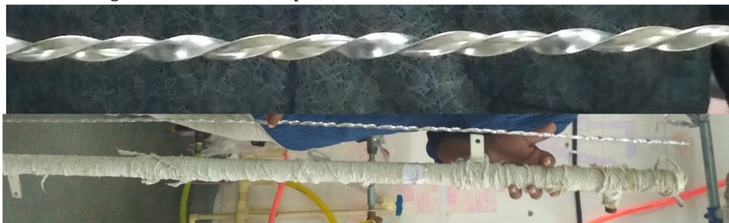
Fig. 2 Twisted tape insert and tube
