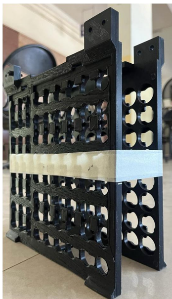
Fig. 9 Casing for Cylindrical Cell
