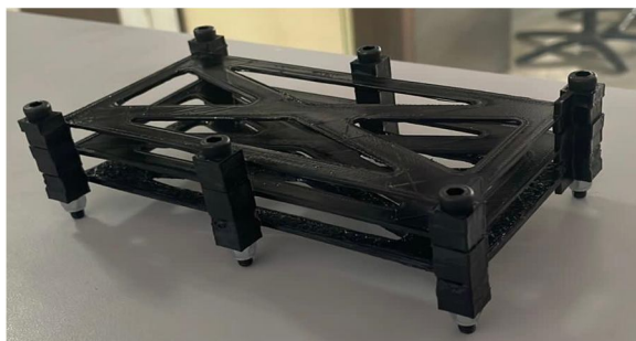
Fig. 8 Casing for pouch cell
