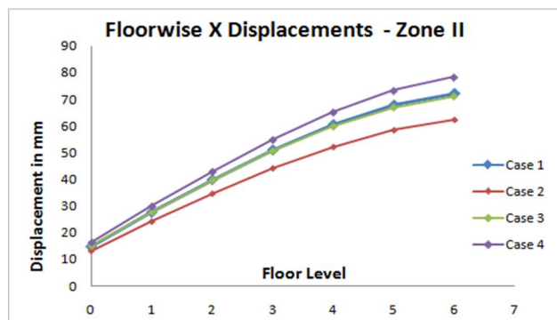
Figure-7 X displacement for Zone II (Corner Column)
