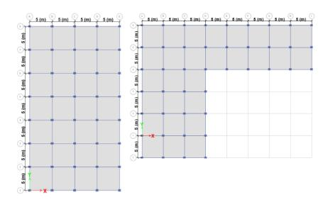
Fig. 1 Column Grid Plan of Symmetric (left) and Asymmetric (Right) RCC Buildings
