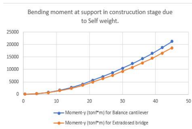
Fig. 10 Comparision of Bending moment at support in construction stage due to Dead Load
