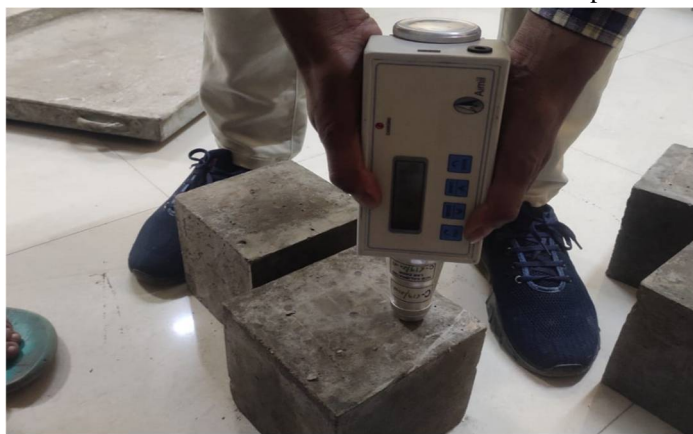
Figure- 4(Rebound Hammer Test)
