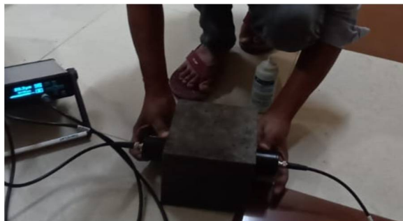
Figure- 6(Ultrasonic Pulse Velocity Test)
