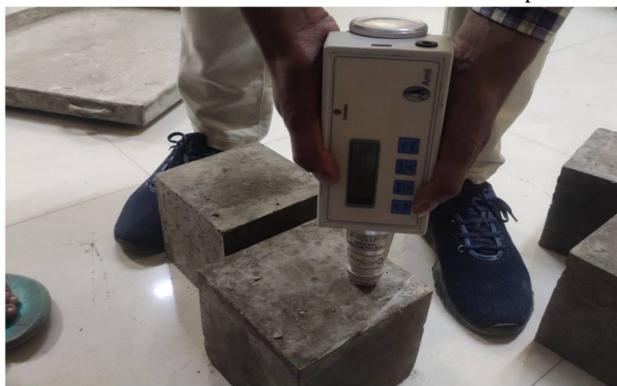
Figure- 4(Rebound Hammer Test)
