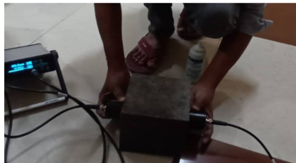
Figure- 6(Ultrasonic Pulse Velocity Test)
