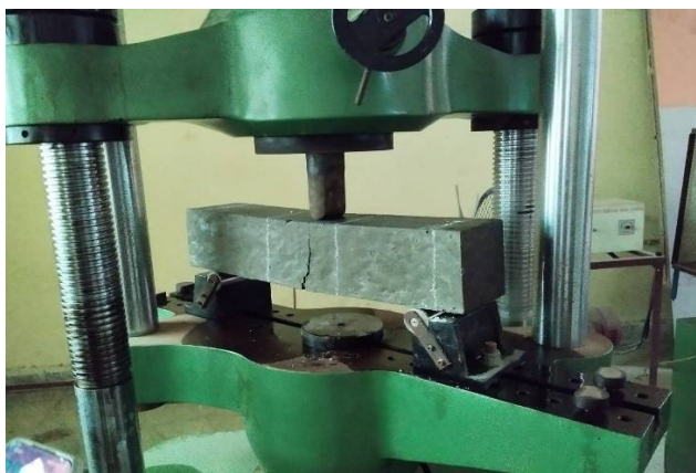
Figure- 3(Flexural Strength Test)
