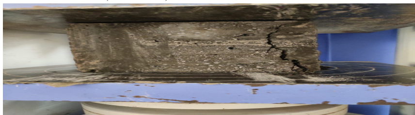
Fig. 3: Performing Compressive Strength Test
