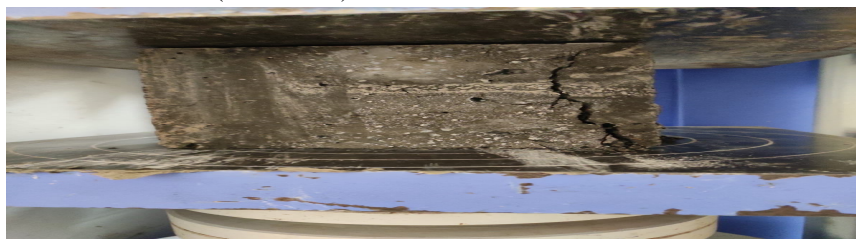
Fig. 3: Performing Compressive Strength Test
