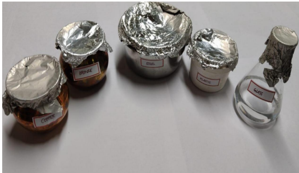
Fig. 1. Various vessels (Copper, Bronze, Plastic, Stainless Steel, and Glass) used for the comparative evaluation of bacterial survival in stored water.
