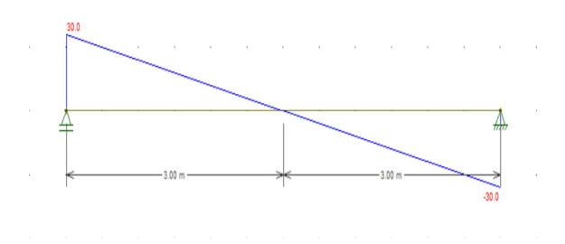
The figure shows the shear force diagram of a simply supported beam with a length of 6.00 m, subjected to a linearly varying distributed load. The shear force varies from +30 kN at the left support to -30 kN at the right support, forming a descending straight line.
