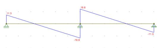
The figure presented shows the shear force diagram of a beam with two simple supports and one double (fixed) support. This configuration defines a first-degree hyperstatic structure, as the number of reactions exceeds the three static equilibrium equations  $(\sum Fx = 0, \sum Fy = 0, \sum M = 0).$
