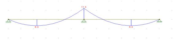
The bending moment diagram corresponds to a continuous beam with two simple supports and one fixed support, characterizing a first-degree hyperstatic structure. The analysis was carried out using Ftool software, which provides internal forces while accounting for deformation compatibility.
