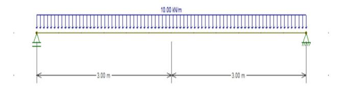
Beam A (Isostatic)
