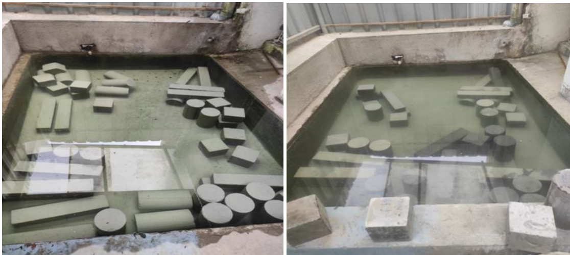
Figure 3: Water Curing of Concrete Specimens
