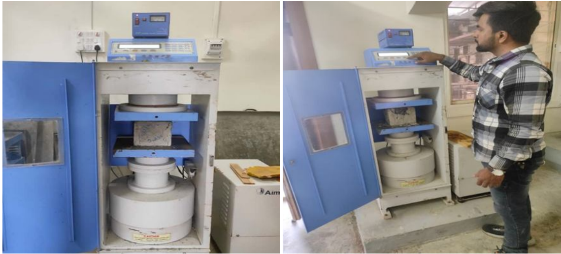
Figure 4: Compressive Strength Test (ACTM)
