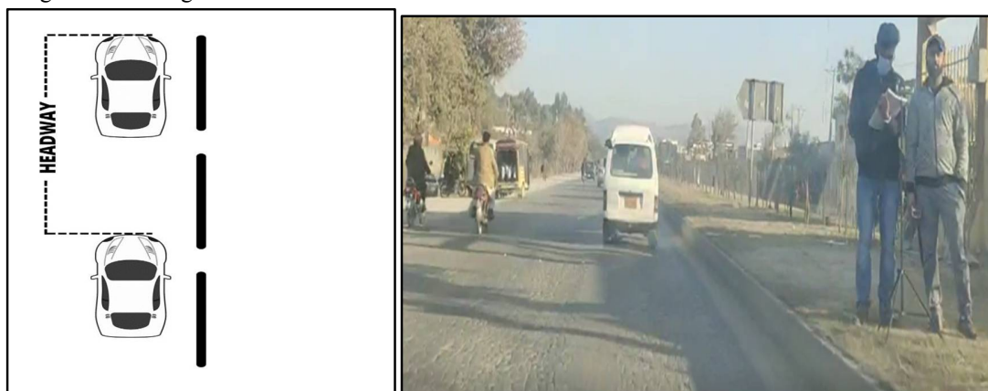
Fig 2: Headway Definition illustration (a), field measurement of headway (b)
