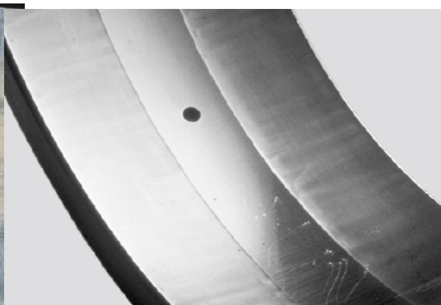
Figure-12: Advanced abrasive wear on the outer ring
