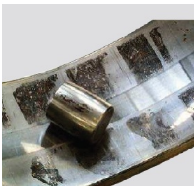
Figure-14: Corrosion on Outer ring
