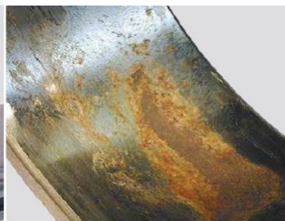
Figure-18: Fretting corrosion on an inner ring due to inadequate shaft seat or shaft bending Figure-19: Fretting corrosion on an inner ring bore resulting from heavy load or inadequate shaft seat
