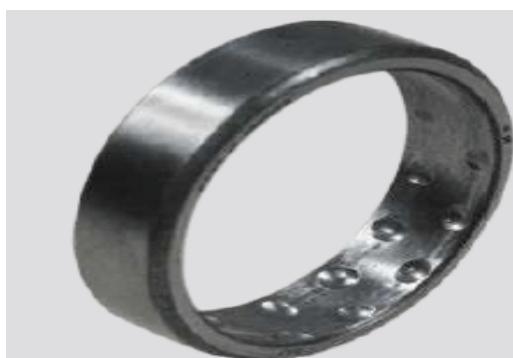
Figure-20: Severe false brinelling on the outer ring raceway of a self-aligning ball bearing
