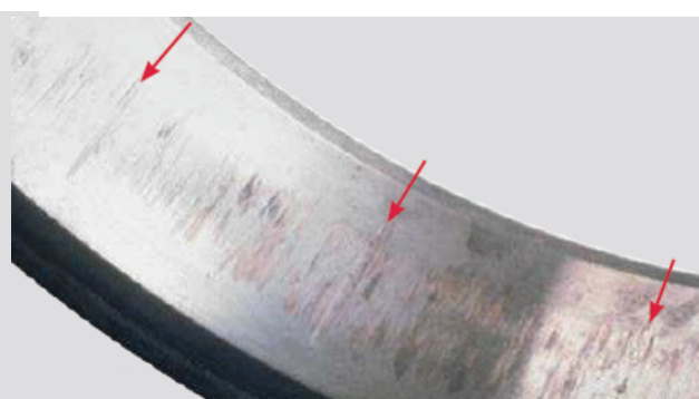
Figure-21: False brinelling ("flutes") on the outer ring raceway
