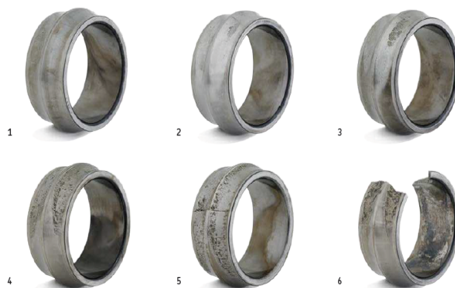
Figure-4: Bearing damage progression
