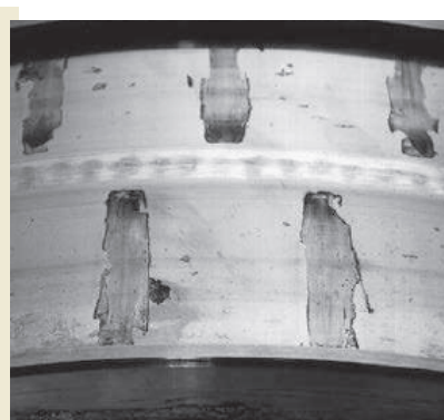
Figure-16: Initial patches of etching at rolling element pitch
