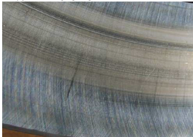
Figure-11: Light abrasive wear on the outer ring
