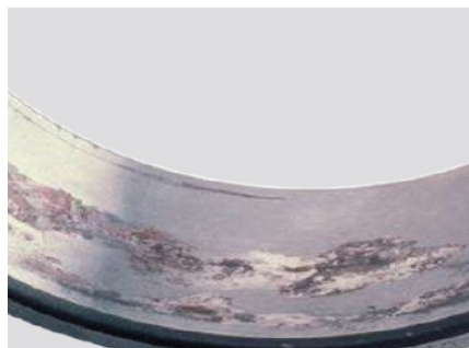
Figure-18: Fretting corrosion on an inner ring due to inadequate shaft seat or shaft bending Figure-19: Fretting corrosion on an inner ring bore resulting from heavy load or inadequate shaft seat
