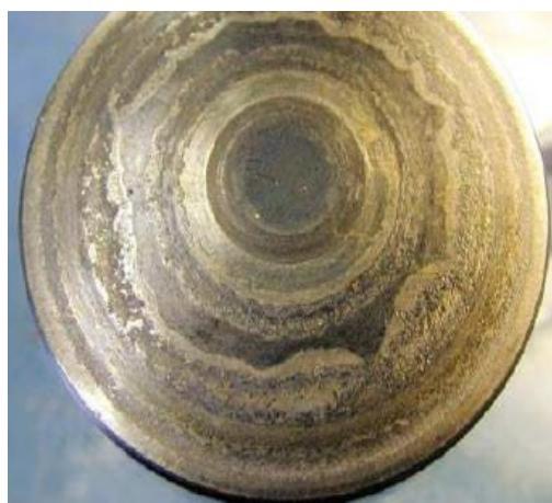
Figure-13: Smearing on a roller thrust face of aspherical roller thrust bearing
