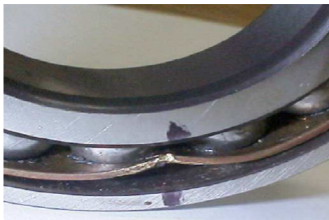
Figure-25: Plastic deformation on the cage of bearing due to poor handling
