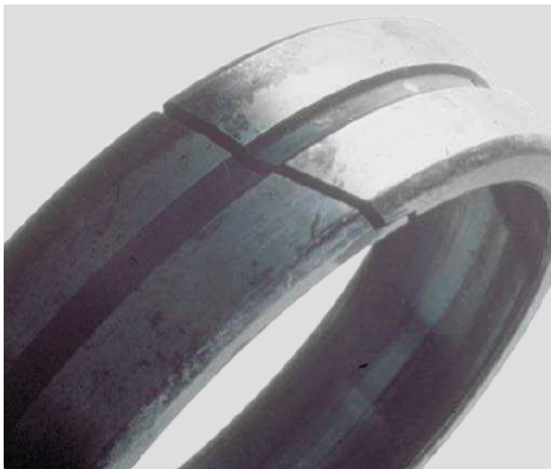
Figure-35: Fatigue fracture of an outer ring of a spherical roller bearing
