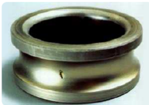
Figure-7: Initial subsurface spalling on the inner ring of a deep groove ball bearing Figure-8: Subsurface spall on an inner ring raceway
