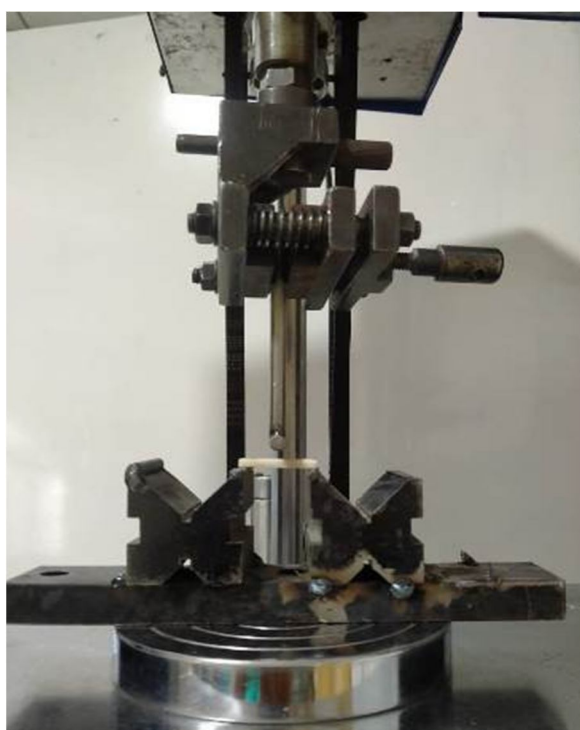
Figure 2. Experimental setup for flexural strength
