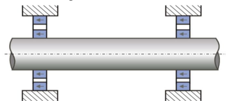
Figure-3: Passive Magnetic Bearing repulsive forces stabilize radial shaft motion
