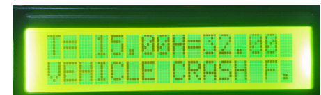
Figure 8: Vehicle Accident detected by front side
