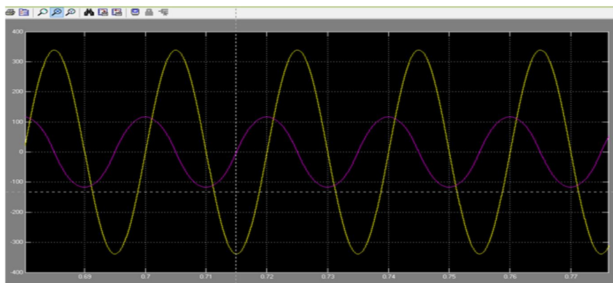
Fig.9 Voltage & Current waveform without STATCOM
