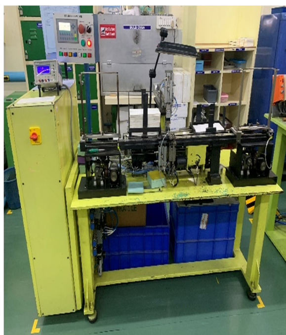
Fig 1.10 Coil unloading machine
