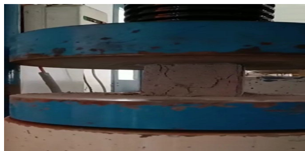
Fig.3 Figure showing AAC block under compression
