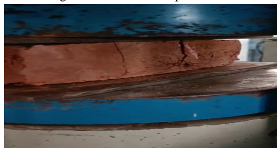
Fig.2 Figure showing Red clay brick under compression
