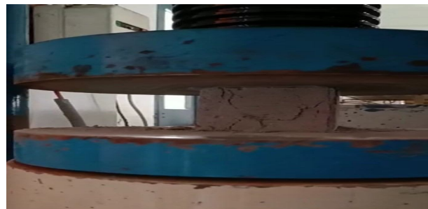
Fig.3 Figure showing AAC block under compression
