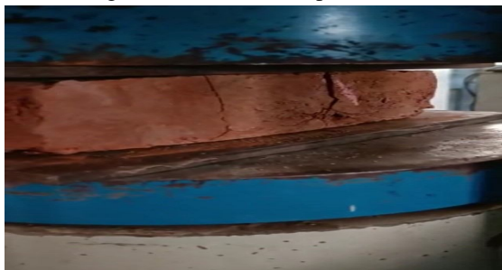
Fig.2 Figure showing Red clay brick under compression
