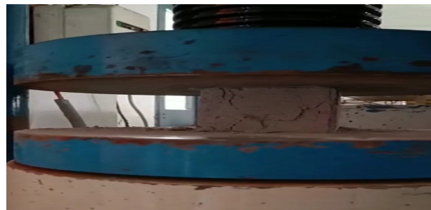
Fig.3 Figure showing AAC block under compression
