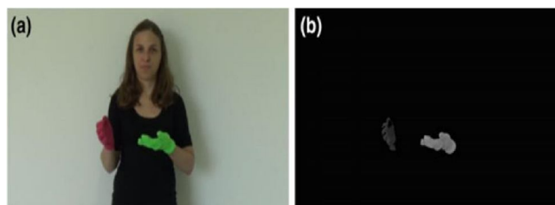
Fig-6 a sample frame from the dataset. b Frame after background removal
