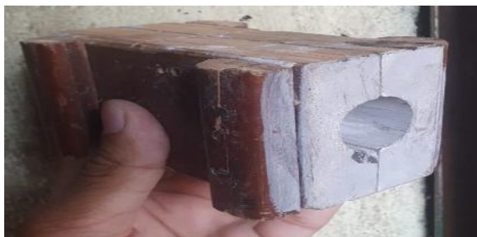
Fig. 2 Core box used for making core
