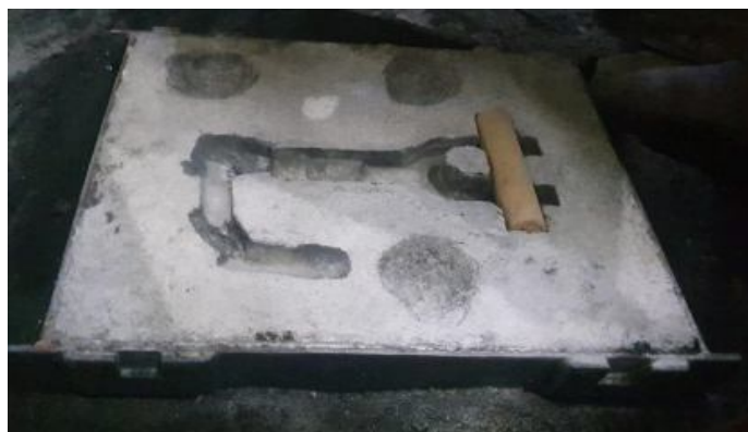
Fig. 3 Drag & Core placed horizontally
