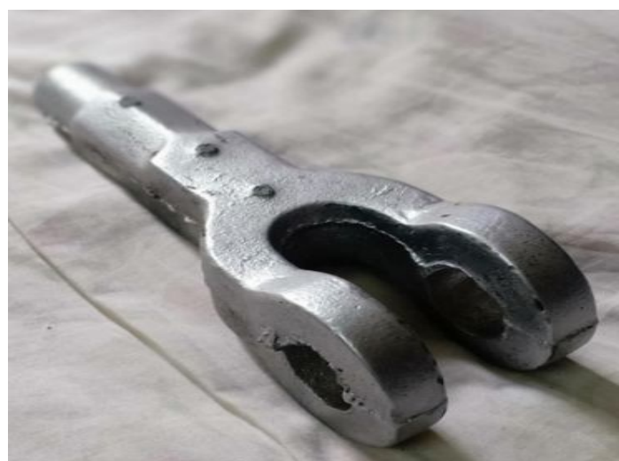
Fig. 12 Defect-free Fork End
