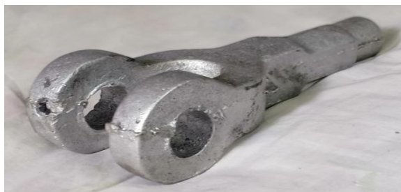
Fig. 13 Defective Fork End
