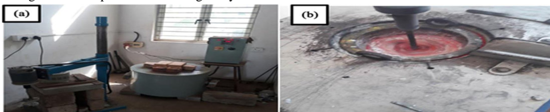
Fig 1: Stir Casting Apparatus and Procedure
