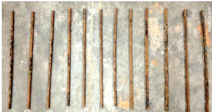
Photograph No. 4.7: Corrosion status of reinforcement in HVFA concrete containing 40%, 50% and 60% fly ash and that containing UFFA
