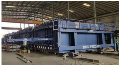
Figure 22: Battery mould for vertical precast wall panels
