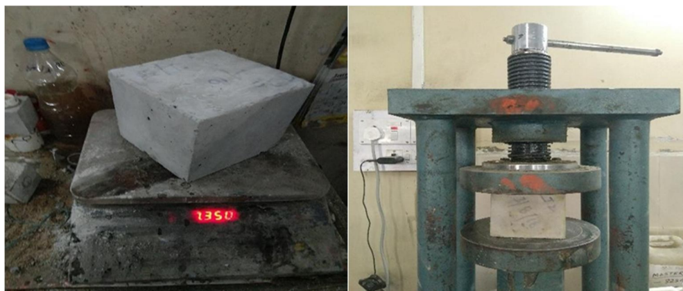
Fig. 1&2 Weight measurement and Compression testing machine
