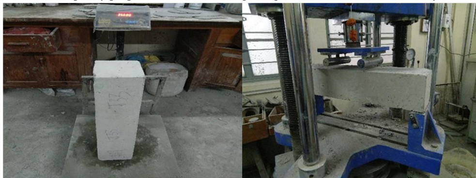
Fig. 4&5 Weight measurement and Flexural testing machine
