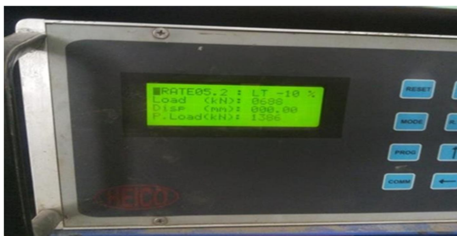
Fig. 3 Compressive load reading in KN
