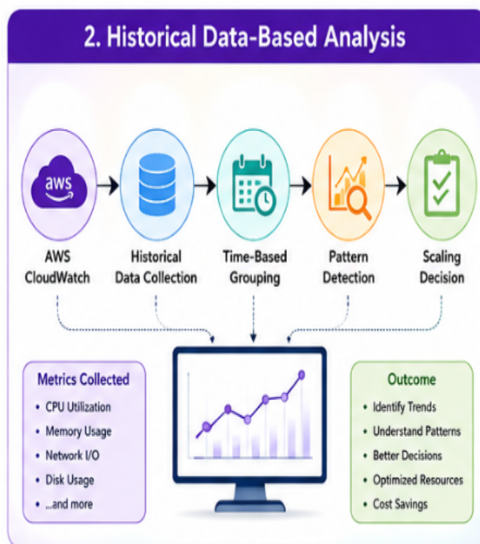
Figure 2 presents the workflow of historical data analysis, beginning with AWS CloudWatch data collection and ending with pattern detection and scaling decision generation.
