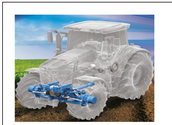
Figure 1. Tractor axle with steering knuckle (schematic)
