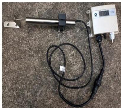
Fig.8: Installation of Linear variable displacement transformer instrument
