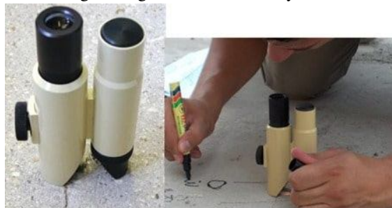
Fig.2: Crack Width Measurement Magnifier
