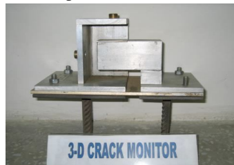
Fig 10 3-D crack monitor (3- dimensional crack monitor)
