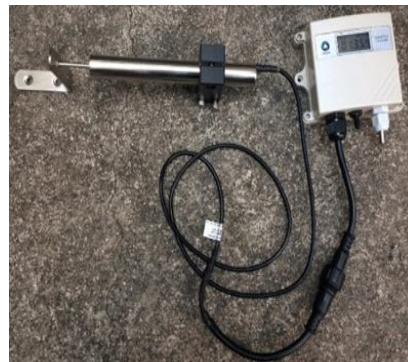
Fig.8: Installation of Linear variable displacement transformer instrument
