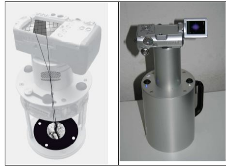
Fig 9 New digital crack monitoring device DRS
