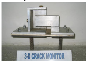
Fig 10 3-D crack monitor (3- dimensional crack monitor)
