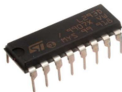
Fig. 9. Motor Driver IC (L293D)
