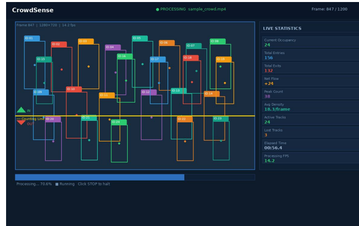
Figure 3: Real-Time Crowd Detection and Tracking Interface with Live Analytics
