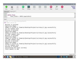
Above is output from the Raspberry Pi's screen. Our system is working completely fine and the way we wanted it to work. With each time when the button is pressed it takes the images, predict it and store it in the list and after pressing the second button it's giving out the total amount as 360 which is also correct.
