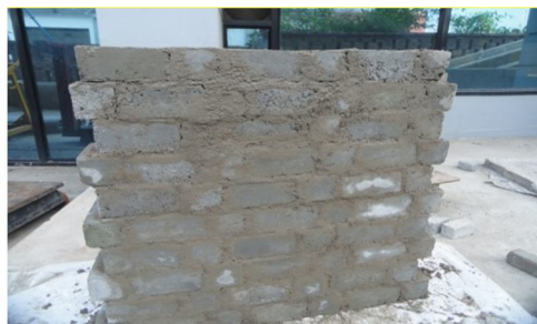
Fig.2 Preparation of test specimen in Modified rat-trap bond
