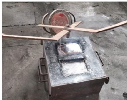
Fig 1: Pouring of molten aluminium
