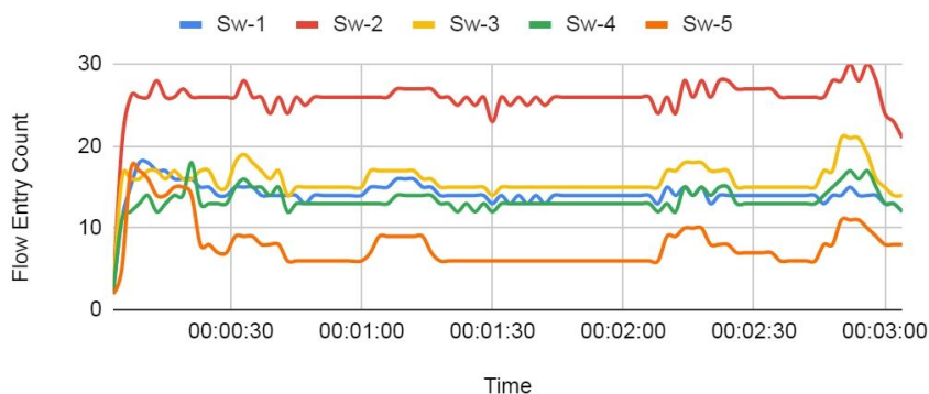
Fig. 9 (b) Flow Table Utilisation of All Switches with DDoSMitigator
