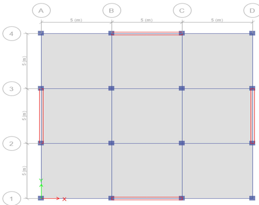
Fig. 4: Plan view of model (i) with shear wall at centre
