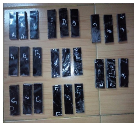
Figure 4.4 prepared Water Absorption test specimen
