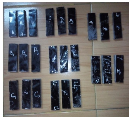
Figure 4.4 prepared Water Absorption test specimen
