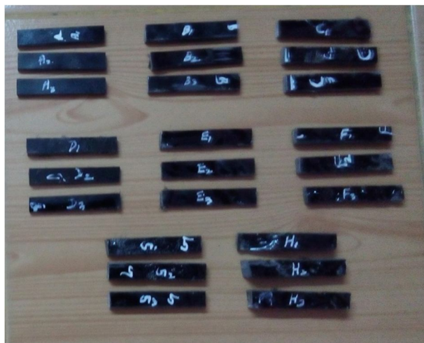
Figure 4.1 Specimens used for performing Impact test.
