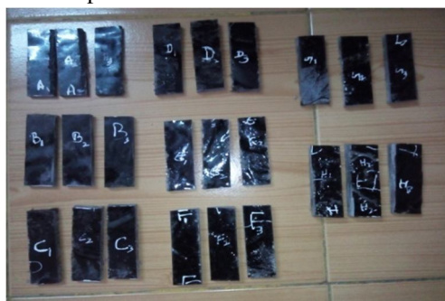
Figure 4.10 Specimens used for Hardness Test
