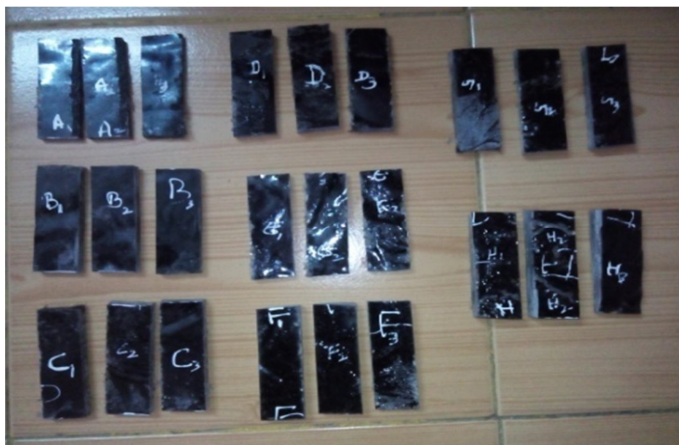
Figure 4.9 Specimens used for determining Density of Composites
