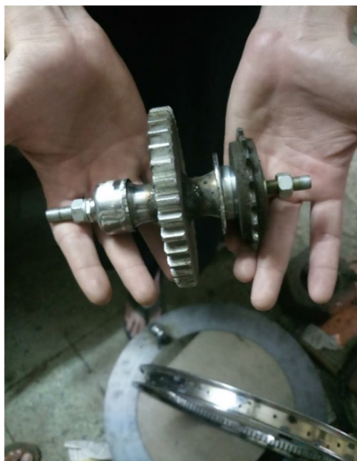
Fig.2: Spur Gear mounted on the hub.
