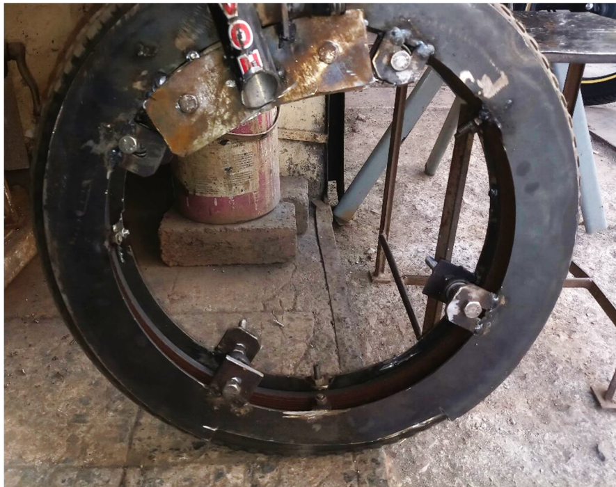
Fig.7: Front wheel mounted on the bicycle frame.
