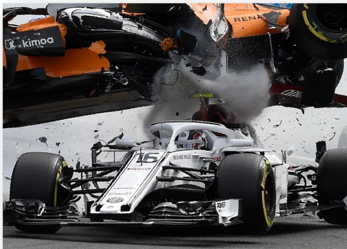
Figure 1 (How halo save driver's head during crash)
