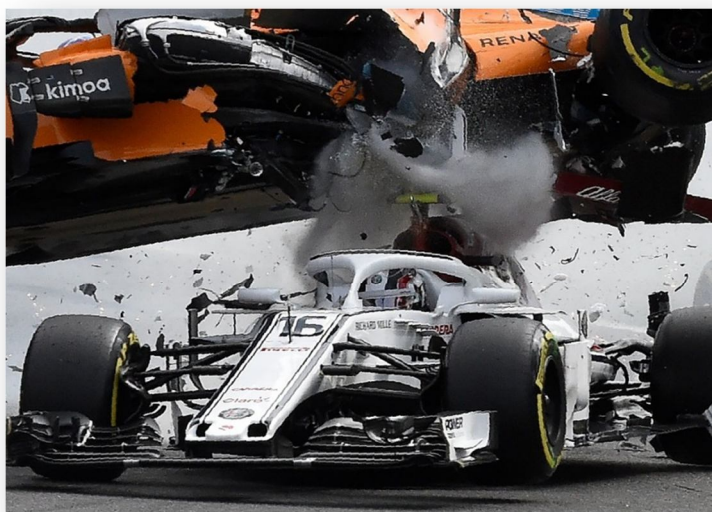
Figure 1 (How halo save driver's head during crash)
