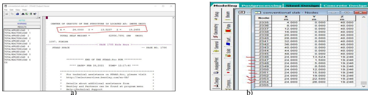
Figure 19: a) Centroid calculation of the building b) centroid for the every floors of building.
