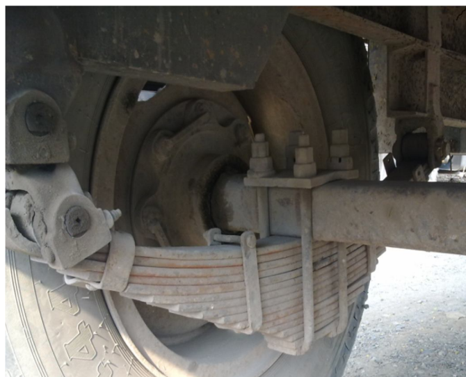
Fig. 1.1: Image of a parabolic semi – elliptic leaf spring
