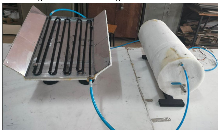
Figure 16 Final experimental setup of Solar water heater
