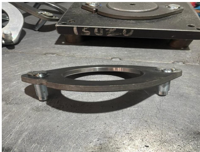
Fig Silencer Nose Ring of SML Isuzu D Max
