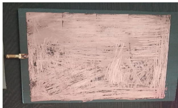
Fig. 4 Antenna built using RT-Duroid 5880 material
