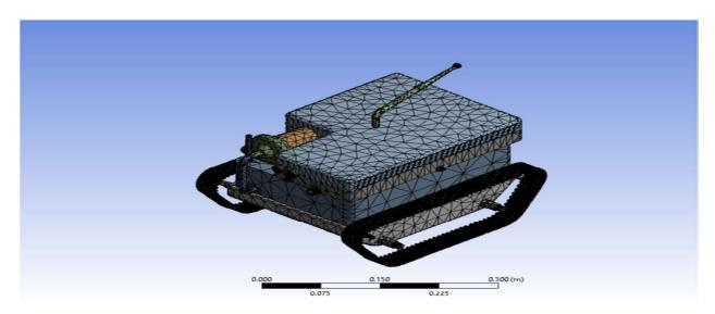
2) Analysis of Mini Fire Fighting Robot: Total deformation is the deformation option that you can see all the deformation results related to your model, in three coordinates (X, Y, Z). Directional: In directional deformation, you can select a coordinate (X, Y, Z) to see the deformation result of your physical model in this direction.
