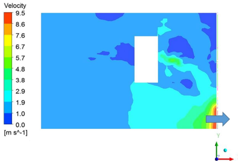
Figure 7: FDS velocity distribution at middle of height
